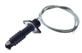
The digital fence sensors will set off an alarm if the wires are cut or if there is an attempt to part the wires in order to gain entry. Each sensor is placed in the middle of a straight run and can detect up to a 100m span of wires. The digital fence system can be combined with an electric fence system. The combination of digital fence and a monitored electric fencing system creates a formidable detection and deterring barrier.
